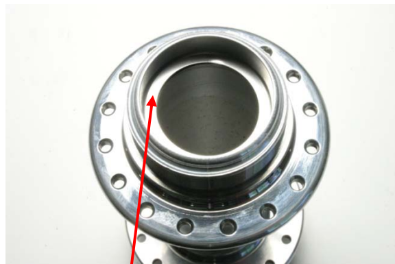
Fig.17 Washers on machined shoulder.
