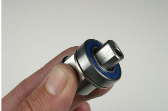
Fig.22 Installing new bearing.
