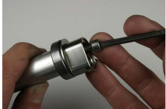
Fig.23 Installing 4mm bolt.
