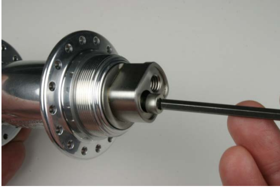
Fig.13 Installing 4mm bolt.
